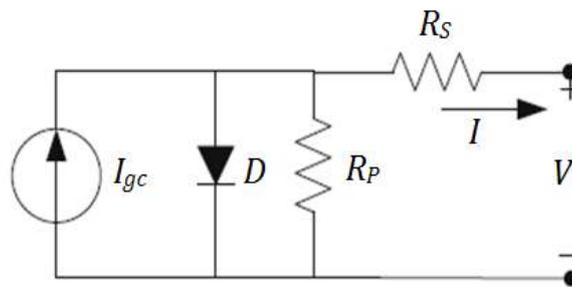
Figure 1. Equivalent circuit diagram of of PV solar cell.
