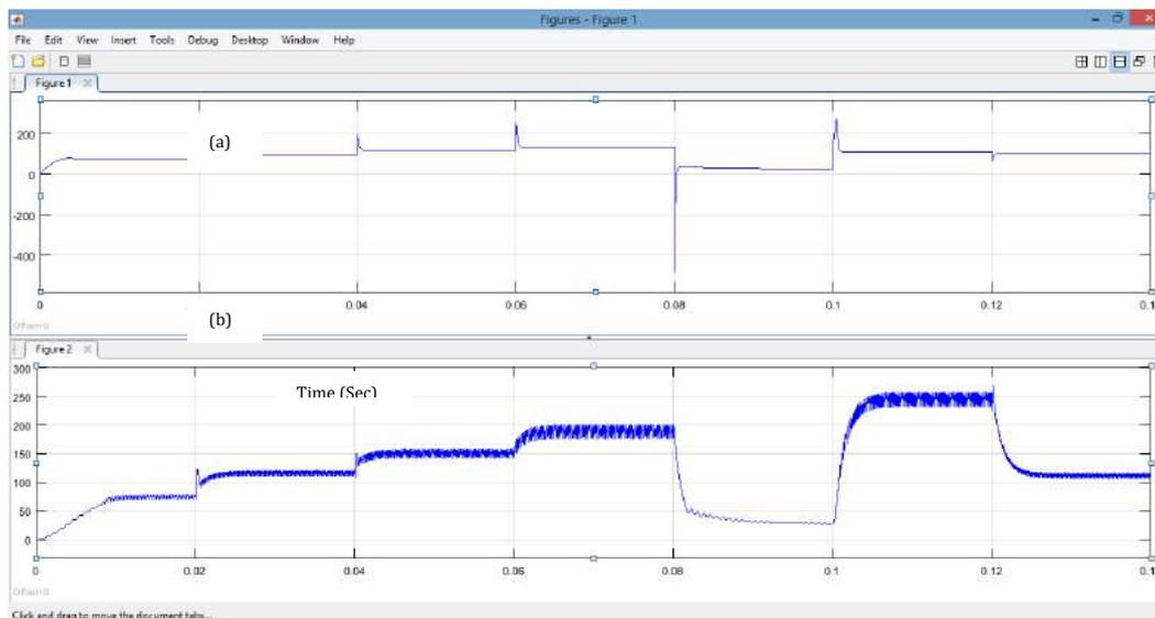
**Figure 25. PV system with (a) the direct connected system compared with (b) ANN MPPT controller with variable irradiation and variable temperature.**
