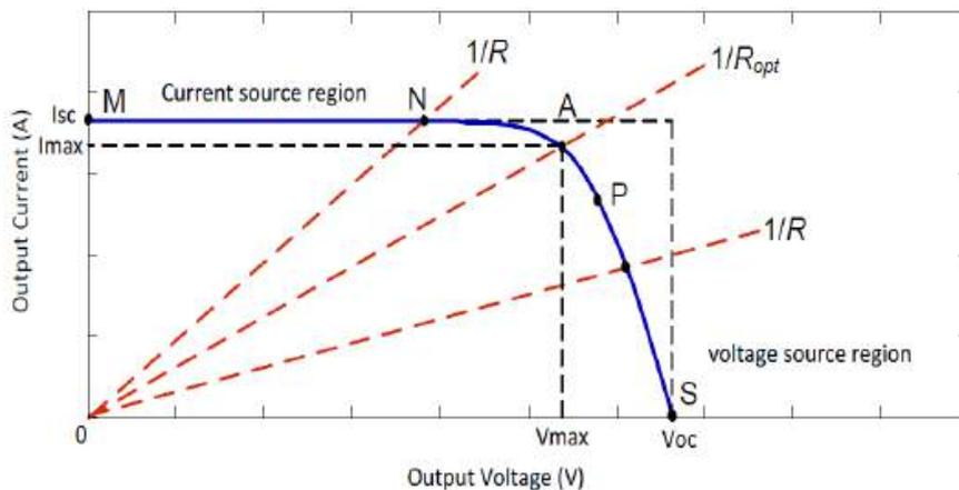
**Figure 7. Intersection of the load characteristic with PV generation curve.**
