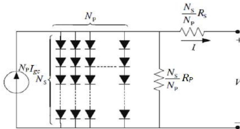
Figure 3. Equivalent circuit diagram of photovoltaic module.
