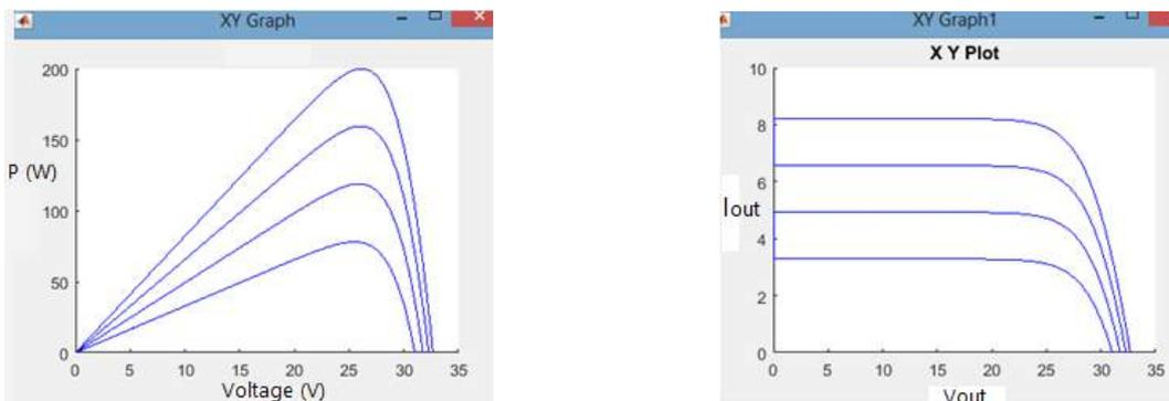
Figure 13. P-V and I-V output characteristics at 25°C.
