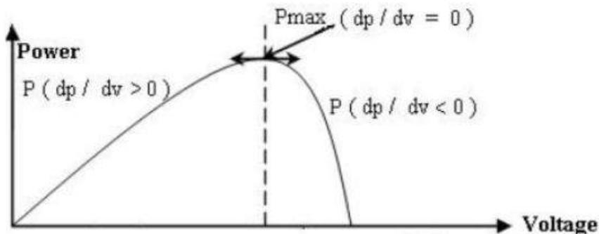
Figure 6. P-V characteristics curve of PV module.
