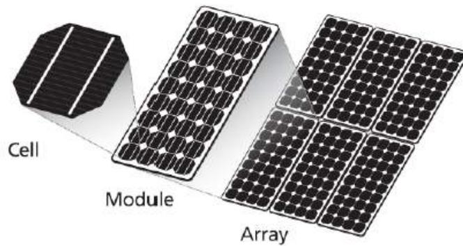
Figure 2. Configuration of photovoltaic cell, module, and array.
