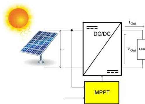
Figure 4. PV with MPPT technique.
