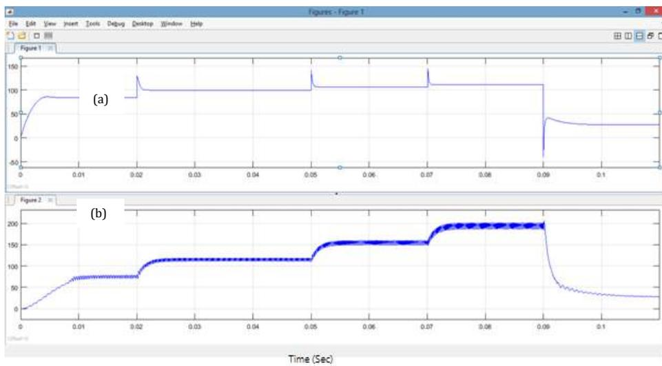
**Figure 24. PV system with (a) the direct connected system compared with (b) ANN MPPT controller with variable irradiation and constant temperature.**
