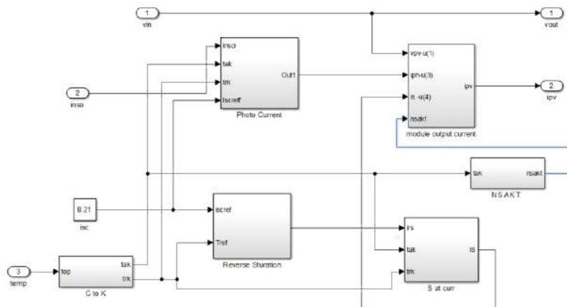
Figure 11. Detailed schematic diagram (sub systems) for the PV module.
