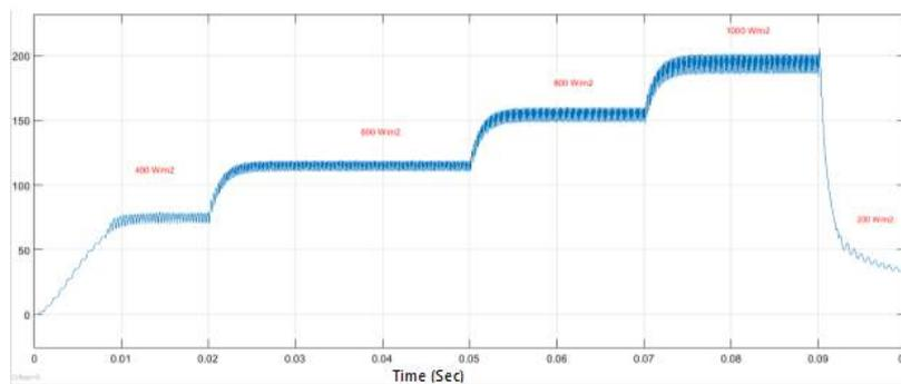
**Figure 22. Output Power for MPPT system with ANN network with variable irradiation and constant temperature (25°C).**
