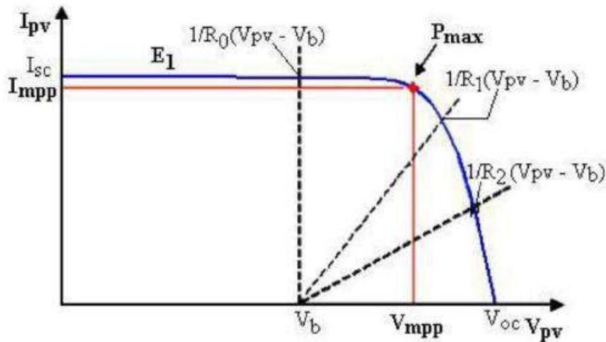
Figure 5. I-V characteristics curve of PV module.
