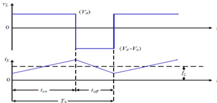
Figure 9. Step-up converter signal form of the VL and IL in continuous conduction mode.
