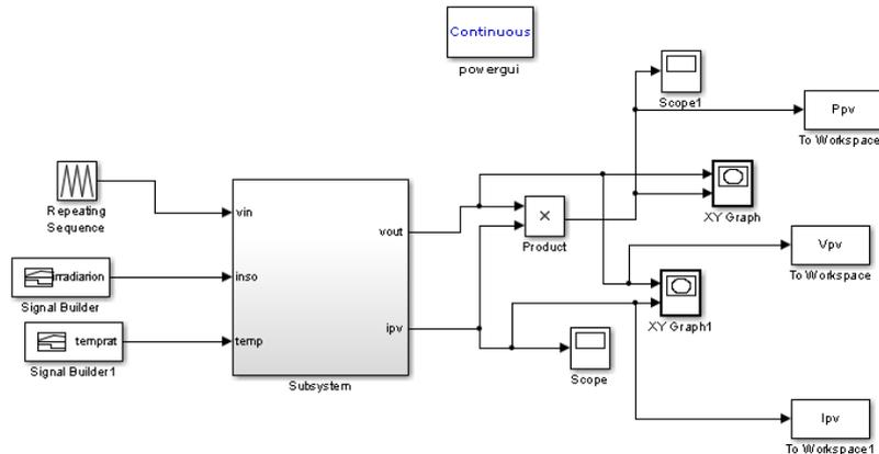
Figure 12. The schematic of PV module.
