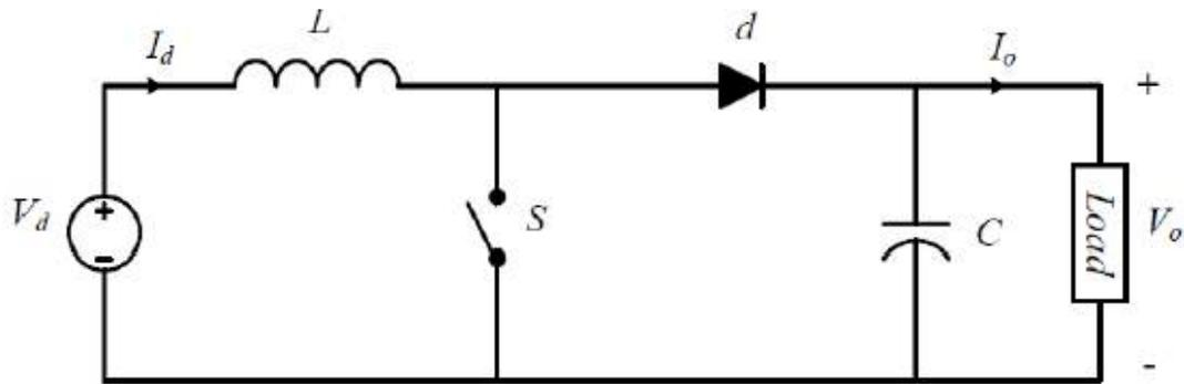
Figure 8. DC-DC step up boost converter.
