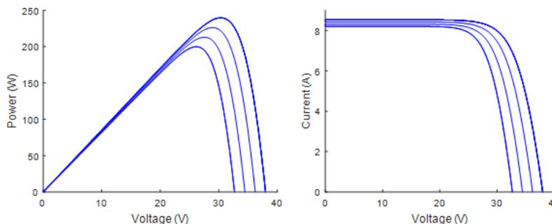
Figure 14. P-V and I-V output of varying temperature and fixed irradiation.
