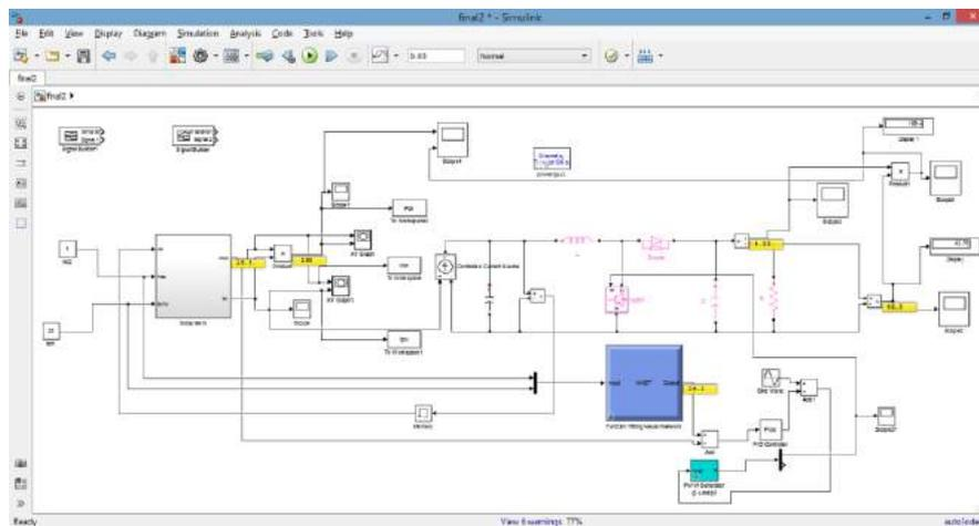
**Figure 21. The complete MPPT system with ANN network.**
